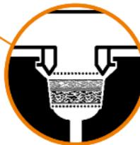
*Filling Chamber partially filled, with Drip Pad placed on top*
