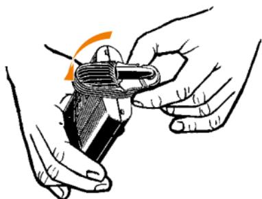
*Removal of Cooling Unit (with Mouthpiece)*
