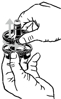
Remove Filling Chamber Cap
