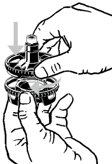
Screw on Filling Chamber Cap
